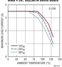
Derating, H-Grade,  $V_{OUT}$  = 2.5V, BIAS = 5V, DC2501A Demo Board
