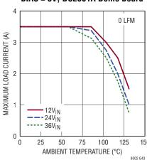
Derating, H-Grade,  $V_{OUT}$  = 2V, BIAS = 5V, DC2501A Demo Board
