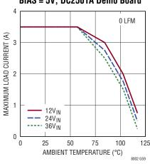
Derating, I-Grade,  $V_{OUT}$  = 1.2V, BIAS = 5V, DC2501A Demo Board
