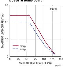
Derating, H-Grade,  $V_{OUT} = -18V$ , BIAS Tied to LTM8002 GND, DC2501A Demo Board
