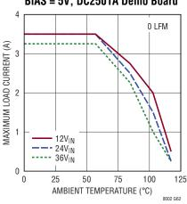
Derating, I-Grade,  $V_{OUT}$  = 2V, BIAS = 5V, DC2501A Demo Board
