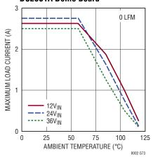
Derating, I-Grade, V<sub>OUT</sub> = -5V, BIAS Tied to LTM8002 GND, DC2501A Demo Board
