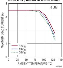
Derating, H-Grade,  $V_{OUT}$  = 1.2V, BIAS = 5V, DC2501A Demo Board
