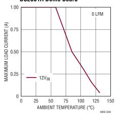
$\begin{array}{l} \text{Derating, I-Grade, V}_{OUT} = 0.97\text{V,} \\ \text{BIAS} = 5\text{V, DC2501A Demo Board} \end{array}$
