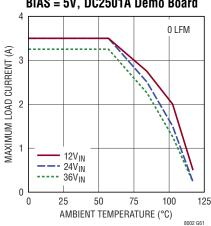
Derating, I-Grade,  $V_{OUT} = 1.8V$ , BIAS = 5V, DC2501A Demo Board
