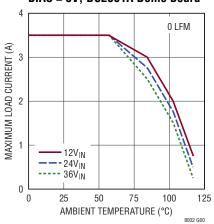
Derating, I-Grade,  $V_{OUT} = 1.5V$ , BIAS = 5V, DC2501A Demo Board
