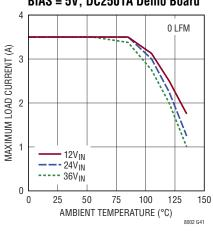
Derating, H-Grade,  $V_{OUT} = 1.5V$ , BIAS = 5V, DC2501A Demo Board
