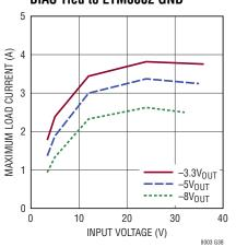
$\begin{array}{l} \text{Maximum Load Current vs V}_{\text{IN}}, \\ \text{BIAS Tied to LTM8002 GND} \end{array}$
