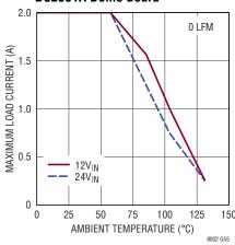
Derating, H-Grade,  $V_{OUT} = -12V$ , BIAS Tied to LTM8002 GND, DC2501A Demo Board
