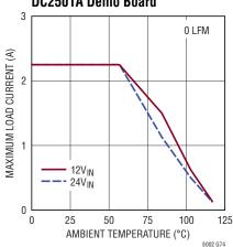
Derating, I-Grade, V<sub>OUT</sub> = -8V, BIAS Tied to LTM8002 GND, DC2501A Demo Board
