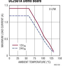
Derating, H-Grade,  $V_{OUT} = -15V$ , BIAS Tied to LTM8002 GND, DC2501A Demo Board
