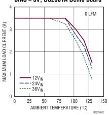
Derating, H-Grade,  $V_{OUT} = 1.8V$ , BIAS = 5V, DC2501A Demo Board
