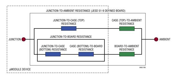
Figure 6. Graphical Representation of the Thermal Resistance Between the Device Junction and Ambient
