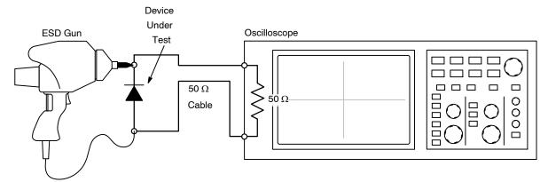
Figure 6. Diagram of ESD Test Setup
