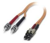
Assembled FO cable, zip cord cable, multi-mode fiberglass  $62.5/125 \mu$ m, OM1, connector: B-FOC (ST)/LC duplex, degree of protection: IP20, for installation in cable ducts or control cabinets
