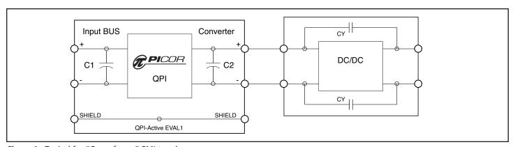
Figure 1 - Typical for "Open-frame" EMI topology
