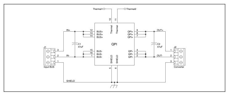
Figure 3 - QPI-X EVAL1 schematic.
