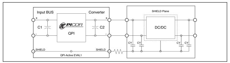
Figure 2 - Typical for "Base-plate" EMI topology
