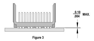
There should be no broken stand-offs along the perimeter of the part (an indication of over-pressing).
