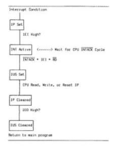
Figure 3. Z8500 Interrupt State Diagram
