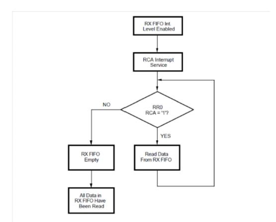
Figure 5. Flowchart of Receive Interrupt Service Routine to Reduce Receive Interrupt Frequencies
