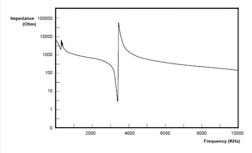
Figure 5. Ceramic Resonator Reactance
