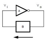
Figure 1. Basic Circuit and Loop Gain
