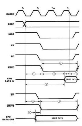
Figure 5. Z80B CPU to Z8500A Peripheral Minimum I/O Cycle Timing
