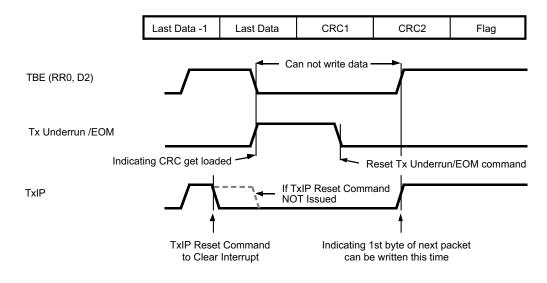
Operation of TBE, Tx Underrun/EOM and TxIP on NMOS/CMOS
