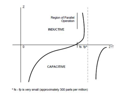
Figure 3. Series vs. Parallel Resonance
