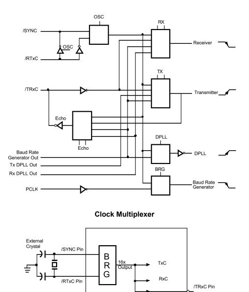
Async Clock Setup Using an External Crystal
