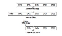
Figure 1. Synchronous Modes of Communication
