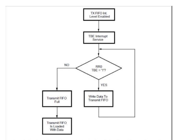
Figure 4. Flowchart of Transmit Interrupt Service Routine to Reduce Transmit Interrupt Frequencies
