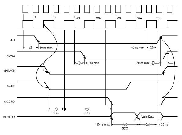
SCC Interrupt Acknowledge Cycle Timing
