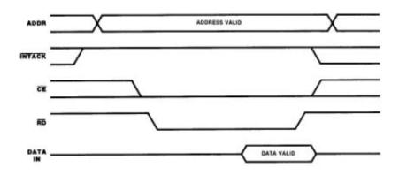
Figure 1. Z8500 Peripheral I/O Read Cycle Timing
