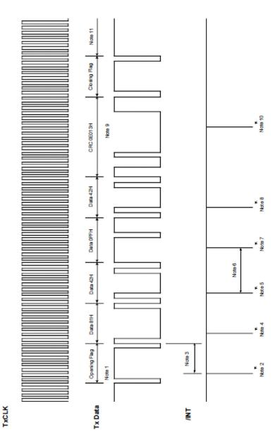
Figure 1. Typical SDLC Transmission Sequence
