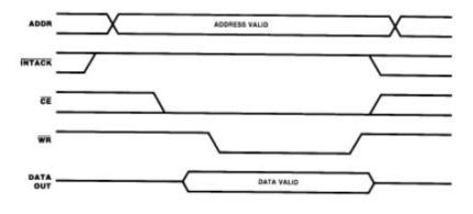
Figure 2. Z8500 Peripheral I/O Write Cycle Timing
