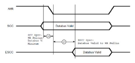
Databus latched after falling edge of WR saves external logic required to delay WR until databus is valid. Typically needed with Intel CPUs.
