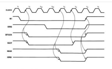
Figure 15. Z80 and Z8500 Peripheral Interrupt Acknowledge Interface Timing
