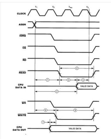
Figure 4. Z80A CPU to Z8500 Peripheral Minimum I/O Cycle Timing
