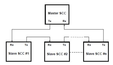
Figure 5. SDLC Loop Mode Configuration
