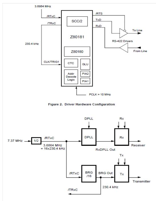
Figure 3. SCC Clocking Scheme
