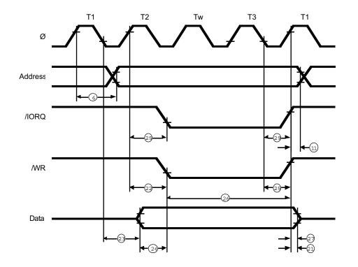
Z180 I/O Write Cycle Timing
