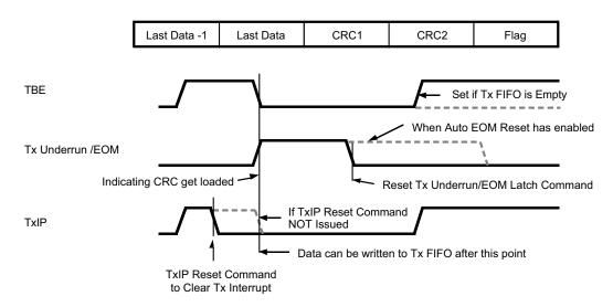
Operation of TBE, Tx Underrun/EOM and TxIP on ESCC
