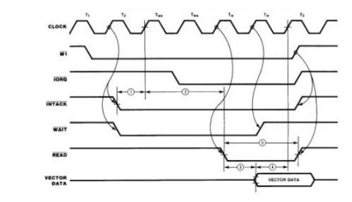
Figure 10. Z80A/Z80B CPU to Z8500/Z8500A Peripheral Interrupt Acknowledge Interface Timing
