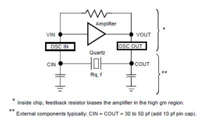
Figure 8. Quartz Oscillator Configuration
