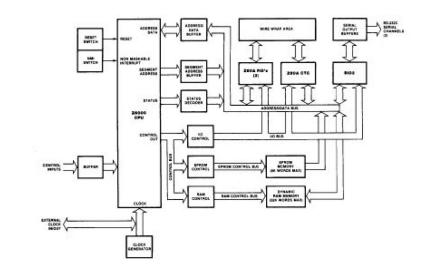
Figure 3. Block Diagram of Z8000 DM
