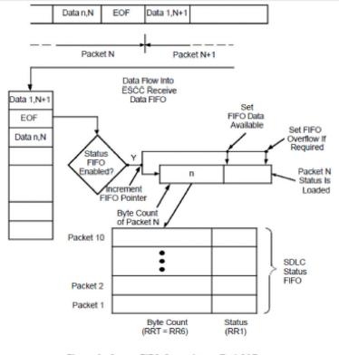
Figure 9. Status FIFO Operation at End Of Frame
